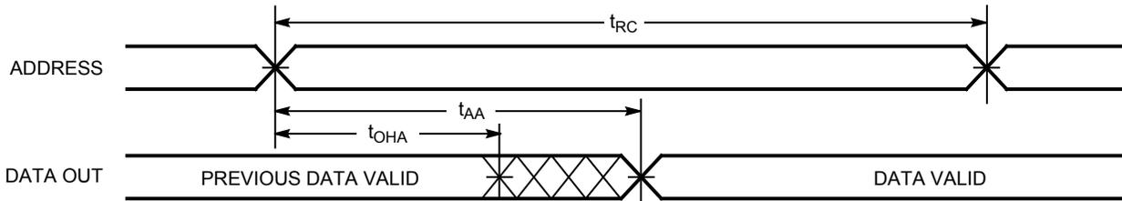
Figure 7. Read Cycle No. 2 ( $\overline{OE}$  Controlled) [23, 24]
